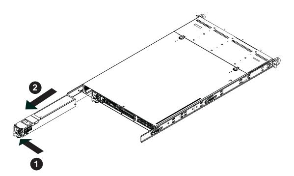
Figure 6-5. Removing/Replacing the Power Supply
